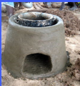
Improved Stove in banco
